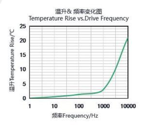
• These temperature rises were measured after applying a sine-wave drive voltage ranging from 0 to 75V at the specified frequency for 10 minutes.
