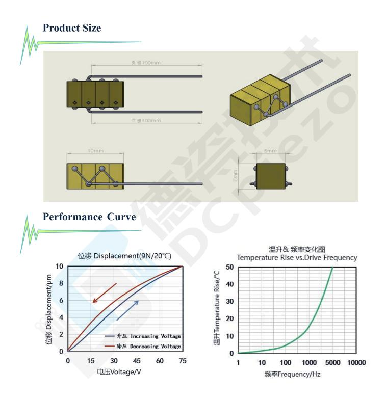
• These temperature rises were measured after applying a sine-wave drive voltage ranging from 0 to 75V at the specified frequency for 10 minutes.
