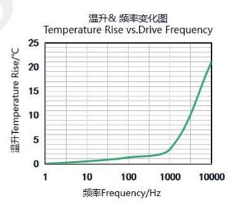
These temperature rises were measured after applying a sine-wave drive voltage ranging from 0 to 100V at the specified frequency for 10 minutes.
