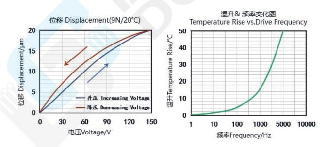
• These temperature rises were measured after applying a sine-wave drive voltage ranging from 0 to 150V at the specified frequency for 10 minutes.
