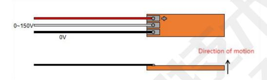
(3) When operating in single-side voltage control mode, avoid simultaneously applying voltage to both the black and red wires. If the voltage difference between the two wires exceeds >150 V, it may damage the actuator.
