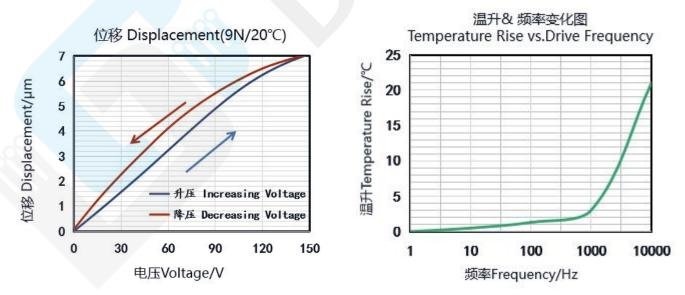
• These temperature rises were measured after applying a sine-wave drive voltage ranging from 0 to 150V at the specified frequency for 10 minutes.
