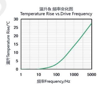
• These temperature rises were measured after applying a sine-wave drive voltage ranging from 0 to 150V at the specified frequency for 10 minutes.
