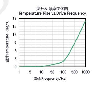
• These temperature rises were measured after applying a sine-wave drive voltage ranging from 0 to 150V at the specified frequency for 10 minutes.
